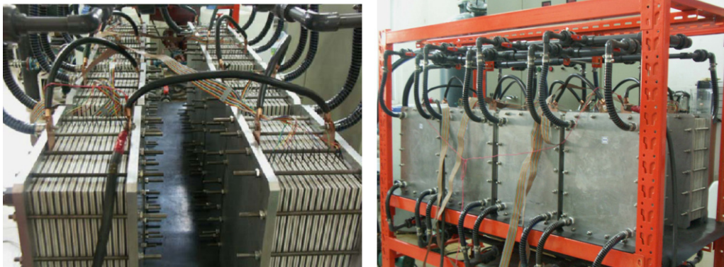
Fig. 5. Photos of 10 kW class VRB cell stack composed of eight 1 kW stack modules with a configuration of 4 \times 2 (serial \times parallel).
